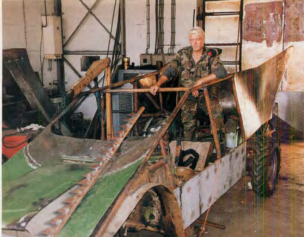
Scorpion, a stripped-down "Mad Max"-inspired design for a fast antitank vehicle. Razor-tooth bars will be welded on either side in front to cut wire while moving cross-country.
